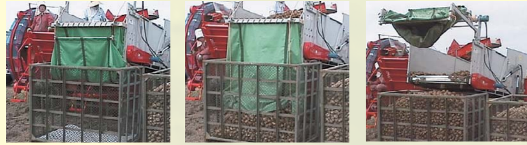
1. Make the chute into a bag and lower it so as to minimize the height from which potatoes will fall. 2. Gradually lower the bag and open the bottom of the chute to evacuate the potatoes. 3. When the container gets full, lift up the chute frame.
